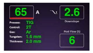
Adjust (2) Post Gas Time and (1) Down Slope to User Preference
